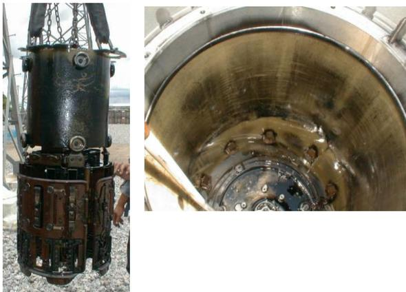
**Fig. 2:** Carbon deposits at the diverter switch insert and the oil compartment
