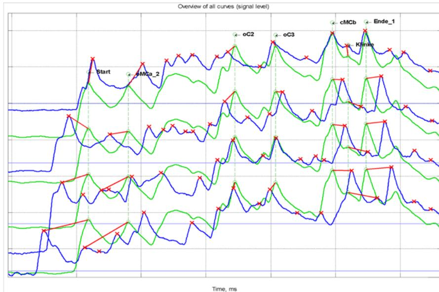
Figure 6: Test curves (blue) and the reference curve (green) for an oil type OLTC. From top to bottom, evolution of the acoustic signature with increasing number of operations.
