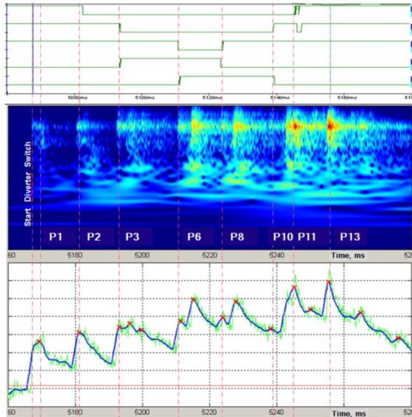
Figure 3: Electrical reference of the contacts breaking and making (at the top), time frequency diagram (in the middle) and resulting envelope (at the bottom) for a diverter switch operation
