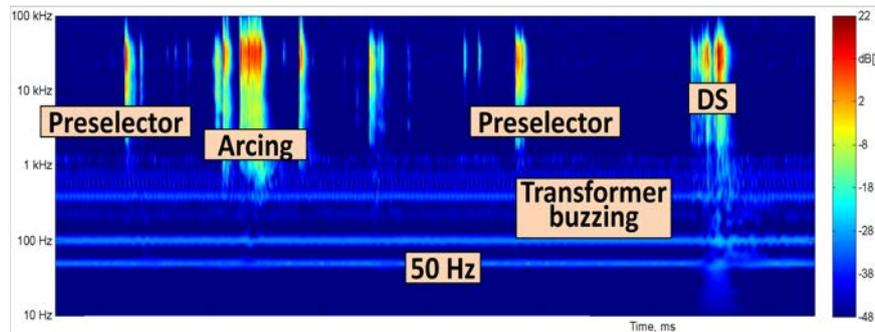
Figure 1: Time frequency representation of an OLTC operation on a transformer in service
