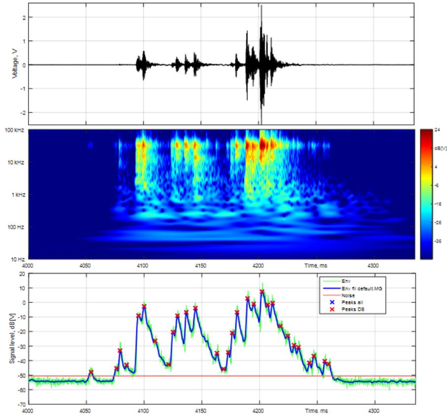
Figure 2: Raw signal of the acceleration sensor (at the top), time frequency diagram (in the middle) and resulting envelope (at the bottom) for a diverter switch operation
