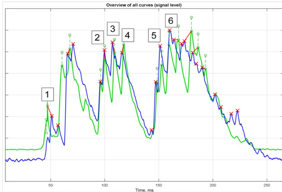
Figure 8: Field example of the analysis of a VACUTAP tap-changer diverter switch
