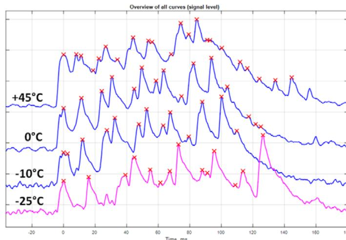
Figure 5: Influence of oil temperature on diverter switch runtime
